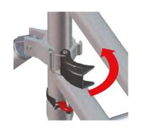
The coupler clamps are used to secure the stabilisers to the tower's vertical tubing. With the clamp jaw open, offer it to the tube. Bring the jaw around the tube and set the buckle on to the hook, then close the clamp arm to lock the stabiliser in position. A similar clamp is fitted to the stabiliser extension leg.
