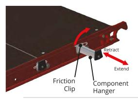
To enable one man to erect MI TOWER products, each hatch is fitted with four component hangers which are stowed (two either side) within the platform's frame. The hangers can be extended when needed and retracted when not.
