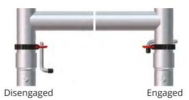
The frame clip's pin locates into a retaining hole in the frames to lock tower sections together when placed one on top of the other. The pin is locked in place by a red tab to ensure that it remains in place. From the disengaged position, pivot the pin / tab to bring the pin horizontal. Insert the pin fully through the retaining hole with its tail pointing down. Next flip the tab vertically to lock the pin in place. Removal is simply a reversal of the fitting sequence.
