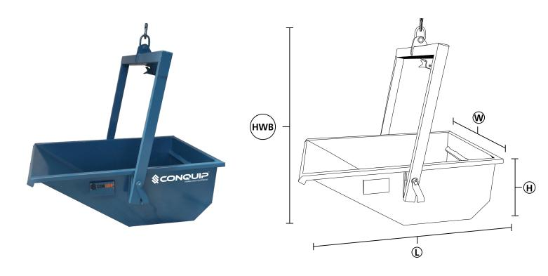
These skips are used for general muck and waste removal. The low loading height and drop down bale arm makes filling very easy. Designed with drop hanger, hook ring and latch for automatic emptying of the skip by the crane operator, without an assistant.
