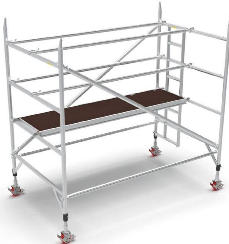
Remove the diagonal brown brace on the non-ladder side of the tower and replace with a 2.4m platform beam. Ensure the top tube of the platform beam is in-line with the top horizontal rungs on the frames and the couplers are fully tightened.
